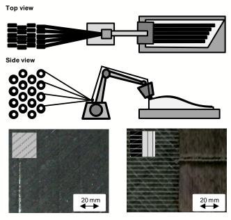
Figure 1: Direct fiber placement and use cases
