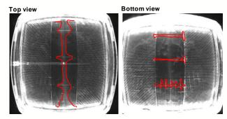
Flowfront progression Figure 3: Influence of stitching in flow-front visualisation of a local reinforced textile (left: top view, right: bottom view)
